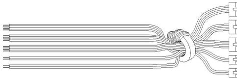
When wiring(Camera, CCTV, Interphone, sensor), please use the core provided in the package to wrap around as shown in the above.
